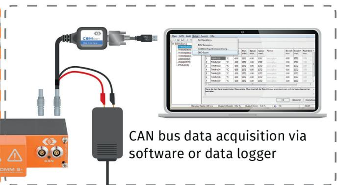
CAN bus data acquisition via software or data logger
