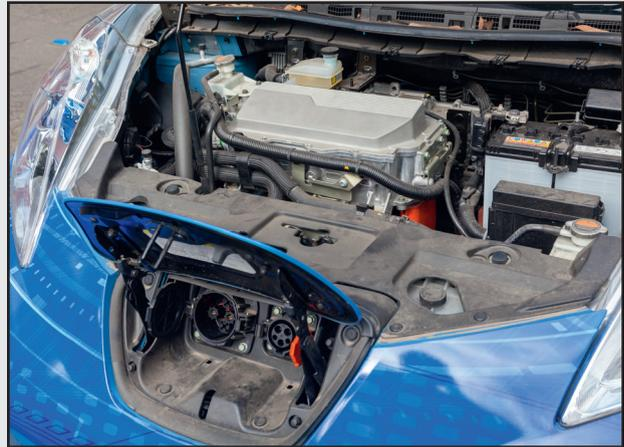
The electric motor as drive element plays a central role, although the term 'electric motor' is not quite correct, as the drive element can also be used as a generator and is also used accordingly in the recuperation.
